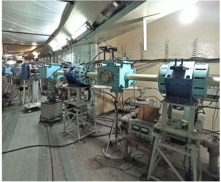
Beam transport path with parallel transfer
